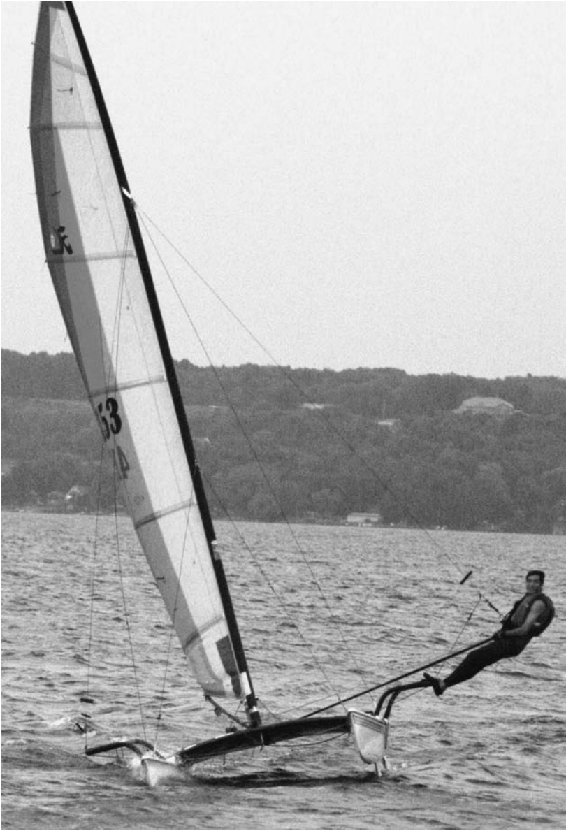
Figure 4.9 The Hobie-17 catamaran can support a large sail and move rapidly because the sailor can supply such a large torque. (Photograph by Richard Olson. With permission.)
