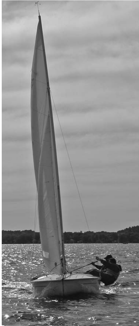
Figure 5.12 A sail resembling the Perfect Blend shape. (Photograph by Sally Snowden. With permission.)
