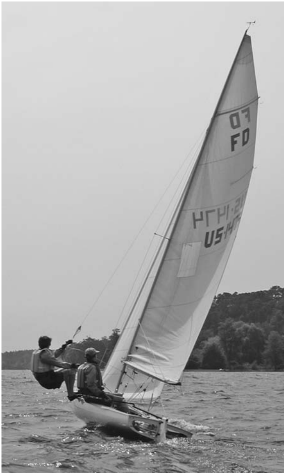
Figure 4.8 The crew on this Flying Dutchman is supported by a cable attached high on the mast. As the wind increases the crew will move out farther. (Photograph by Sally Snowden. With permission.)
