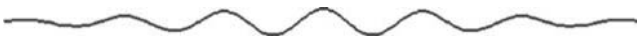
Figure 8.5 A wave packet. This group of waves moves half as fast as the individual peaks.
