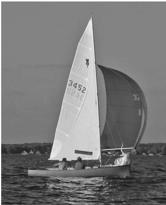
Figure 2.9 The Thistle sailboat sailing approximately downwind. The raised spinnaker and lowered jib change the sail area estimate.
