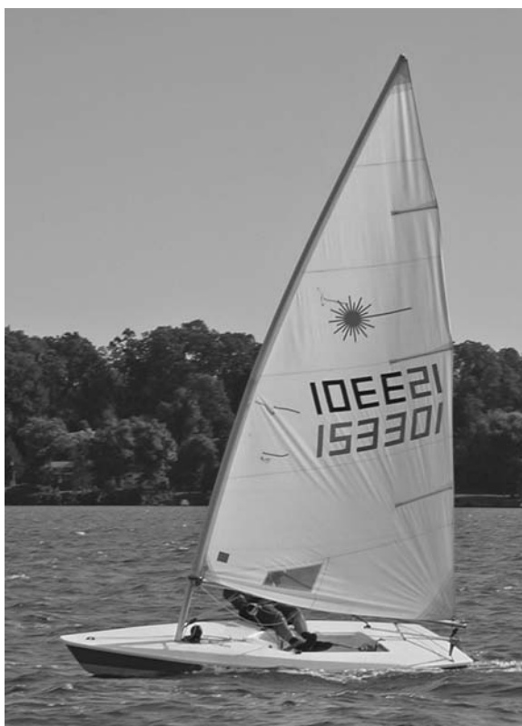
Figure 5.21 Mast bending on a Laser sailboat. (Picture by Sally Snowden. With permission.)
