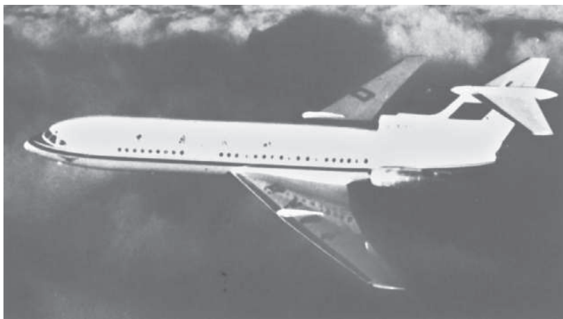
Figure 7.36 Trident illustrating boundary-layer fences on the wing (courtesy of BAE Systems).
