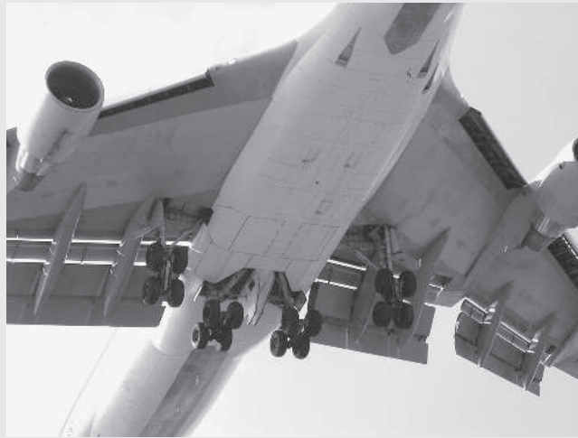
Triple-slotted flap and Krueger flap systems on the Boeing 747 [public domain photo by Adrian Arpingstone]
