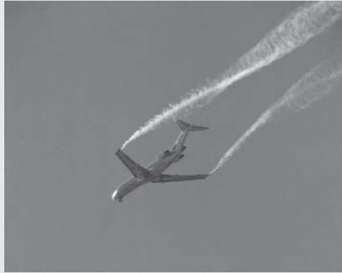
Wing-tip vortices behind a Boeing 727 (photo courtesy of NASA Dryden Flight Research Center)
