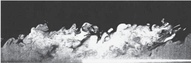
Turbulent boundary layer over a flat plate [Falco (1977)]
