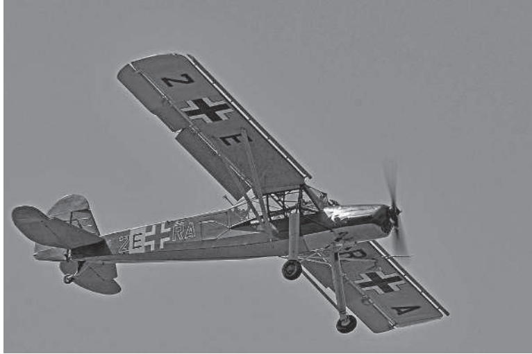
Figure 13.15 Fieseler Storch, Fi 156, showing fixed leading-edge slots and hinged trailing edge (courtesy of David Schultz Photography).
