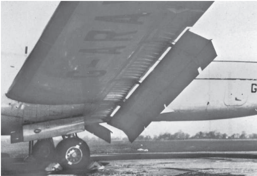
Figure 13.2 Multi-element, high-lift configurations: (a) Fowler flap; (b) double-slotted flap; (c) leading-edge slat, Krueger leading-edge flap, spoiler, and triple-slotted flaps (representative of Boeing 727 wing section); (d) Fowler flaps on the HS 748 (courtesy of BAE Systems).
