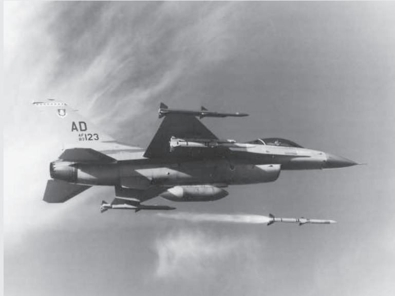
F-16 firing an AMRAAM missile (U.S. Air Force photo by Staff Sgt. Eric T. Sheller)
