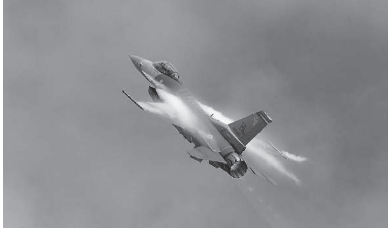
Figure 13.20 Strake vortex system on an F-16 (U.S. Air Force photo by Josh Plueger).
