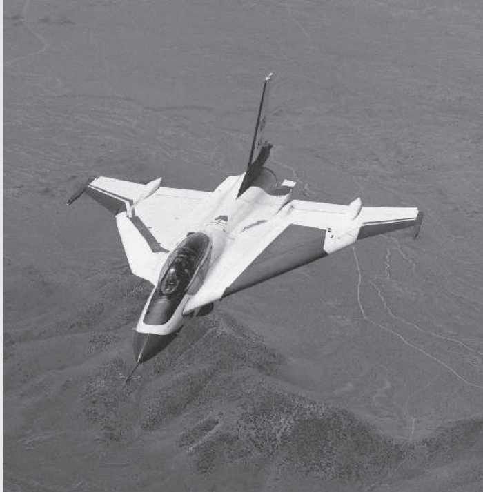
F-16XL with laminar flow glove on port wing (photo courtesy of NASA Dryden Flight Research Center)
