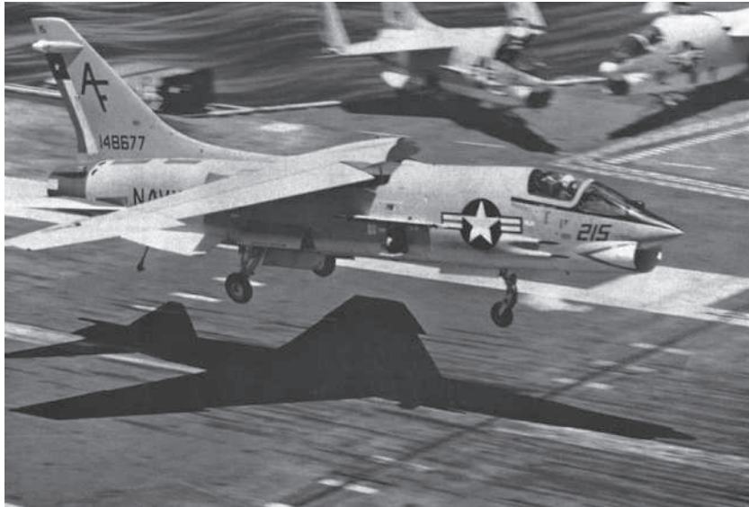
Figure 13.6 Chance-Vought F-8H Crusader showing incidence for the wing during landing (U.S. Navy photo by PH2. P. Staley)
