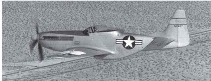
Figure 6.14 Restored NACA P-51 with laminar flow airfoil sections [courtesy of NASA Dryden Flight Research Center].
