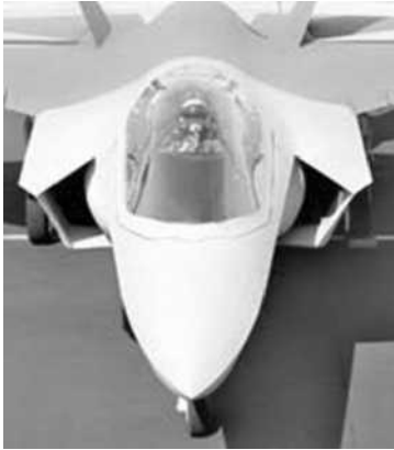
Figure 13.52 The JSF diverterless supersonic inlet (photo courtesy of Lockheed Martin).
