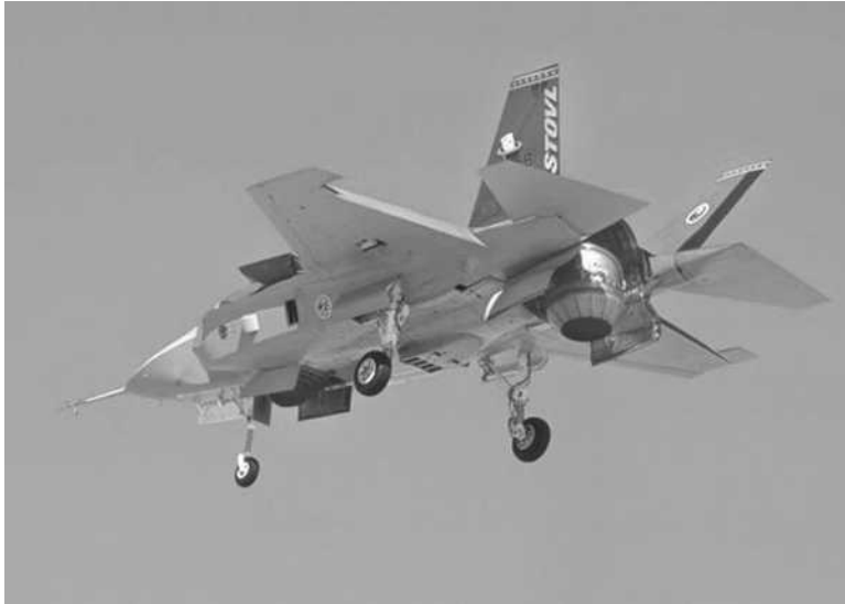
Figure 13.53 The Lockheed Martin X-35B approaching landing in STOVL configuration [from Bucholz (2002); photo courtesy of Lockheed Martin].
