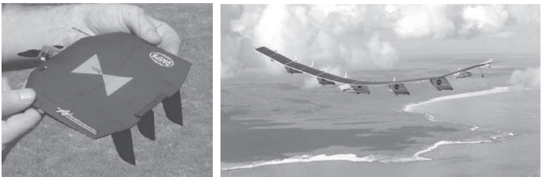
Figure 6.15 Candidate laminar-flow airfoil aircraft: Black Widow Micro UAV (left) and Helios high-altitude solar-powered aircraft (right) [Black Widow from Grasmeyer and Keennon (2001), courtesy of AeroVironment, Inc.; Helios courtesy of NASA Dryden Flight Research Center].
