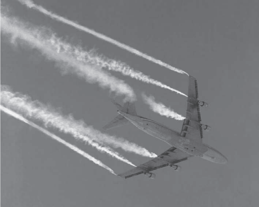
Figure 7.4 ( Continued ) (b) Streamwise vorticity shedding along the trailing edge of a Boeing 747 rolling up into wing-tip vortices (courtesy of NASA Dryden Flight Research Center).
