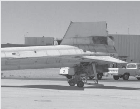
X-15A-2 after landing: notice charring on lower pylon and speed brake on vertical tail (courtesy of NASA Dryden Flight Research Center)
