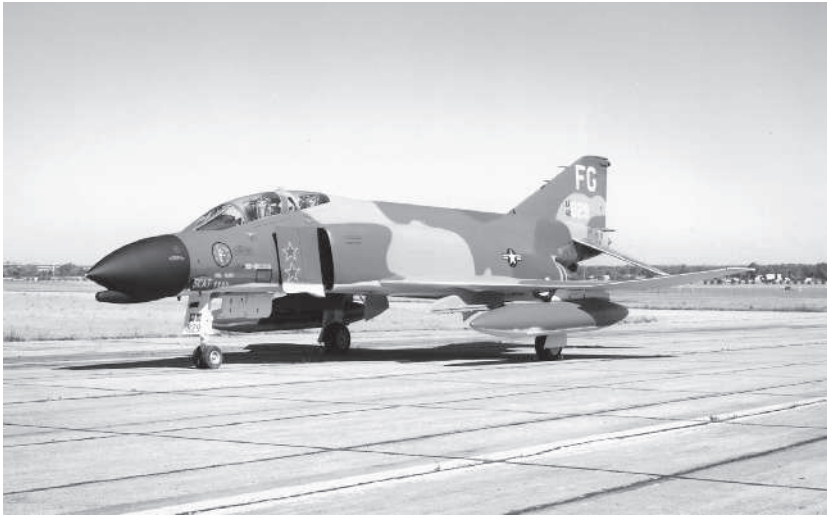
a) F-4C which was flown at 35,000 ft in level acceleration; W = 38,924 lb with 4 AIM-7 missiles (US Air Force photo)
