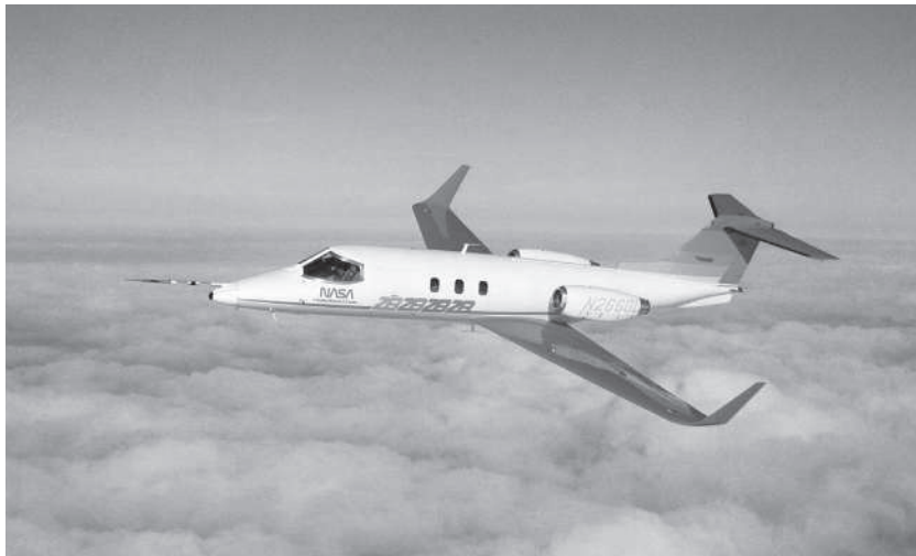
Figure 13.24 Gates Learjet Model 28/29, the Longhorn, illustrating use of winglets (Image provided courtesy of Bombardier Inc.).
