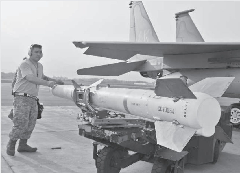
AMRAAM being loaded onto an F-15 (U.S. Air Force photo by Senior Airman Laura Turner)
