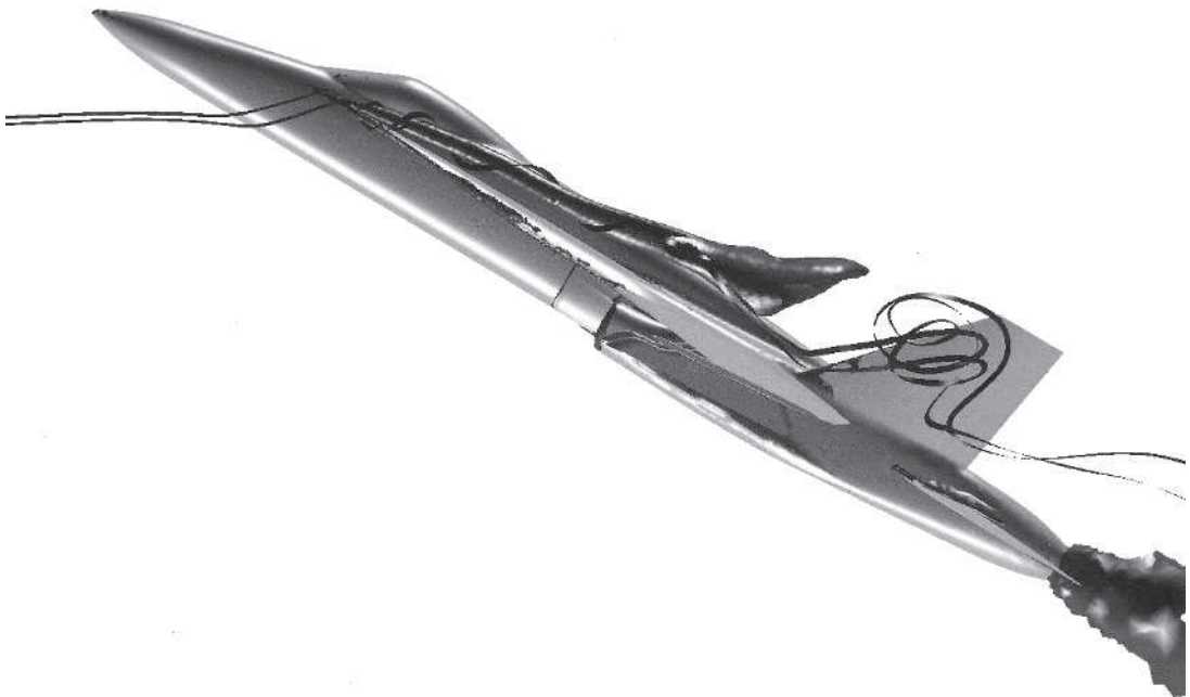
Figure 7.54 Flow-field computations for an F-18C at an angle of attack of 32^\circ , M_\infty = 0.25 , Re_L = 15 \times 10^6 [provided by Wurtzler and Tomaro (1999)].
