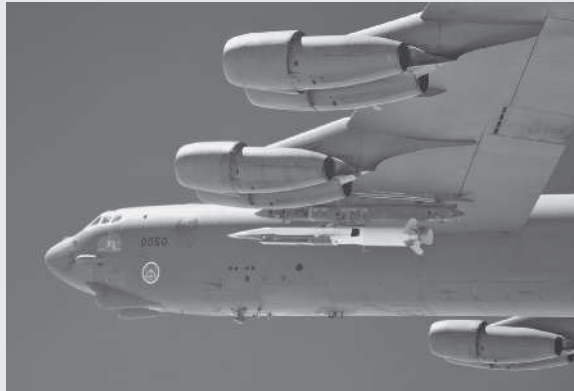
A B-52 carries an X-51A Waverider prior to the scramjet’s first hypersonic flight test (U.S. Air Force photo)
