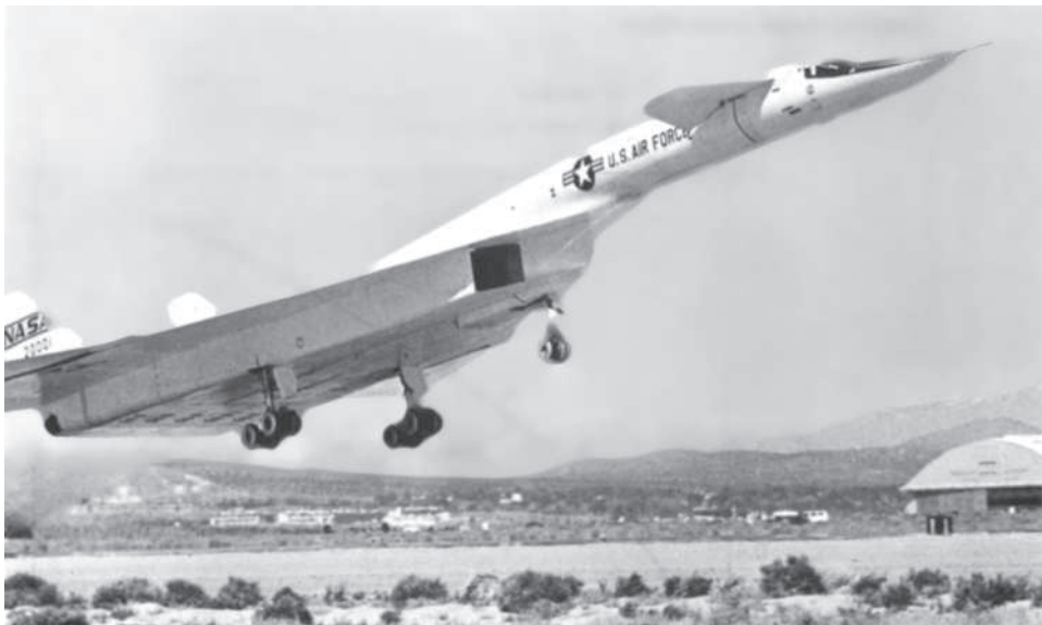
Figure 7.50 North American XB-70 illustrating the use of canards (photo courtesy of NASA).
