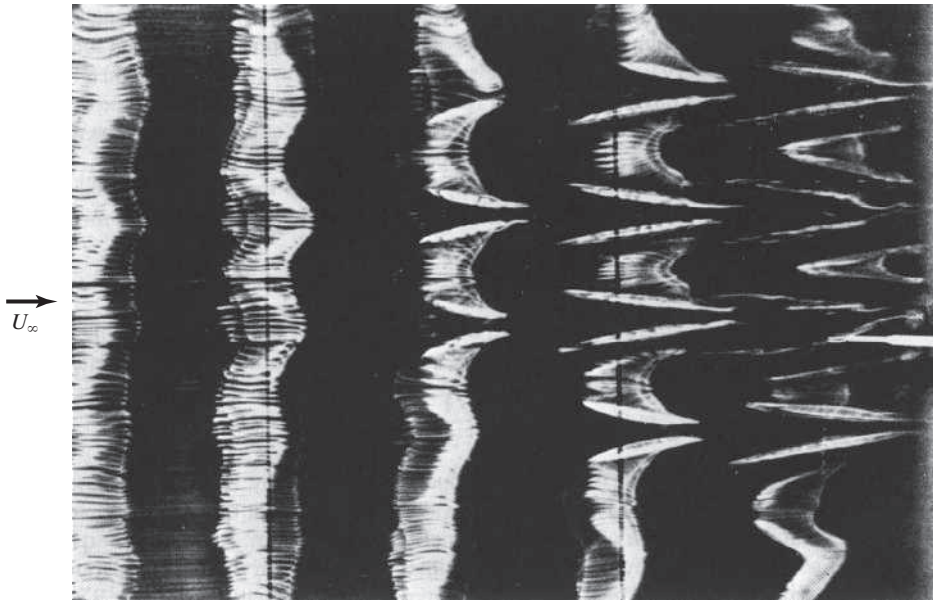
Figure 4.13 Flow visualization of the transition process on a flat plate (photograph supplied by A. S. W. Thomas, Lockheed Aeronautical Systems Company, Georgia Division).
