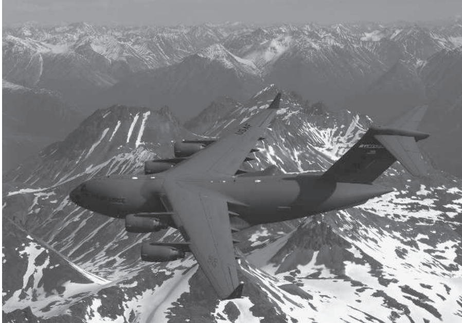
Figure 5.1 The wing of the C-17 (which includes supercritical airfoil sections, leading-edge devices, blown flaps, and wing-tip devices) represents the complexity of a modern airplane wing system (U.S. Air Force photo by Tech Sgt. Keith Brown).
