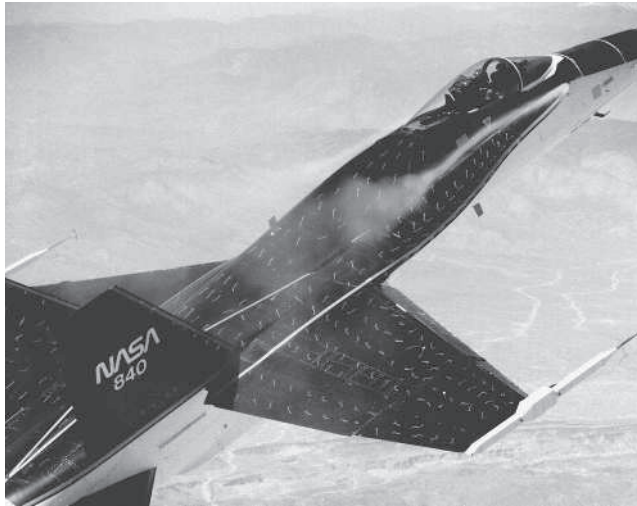
Figure 6.31 F-18 HARV at \alpha = 30^\circ with smoke and tuft visualization (courtesy of NASA Dryden Flight Research Center).
