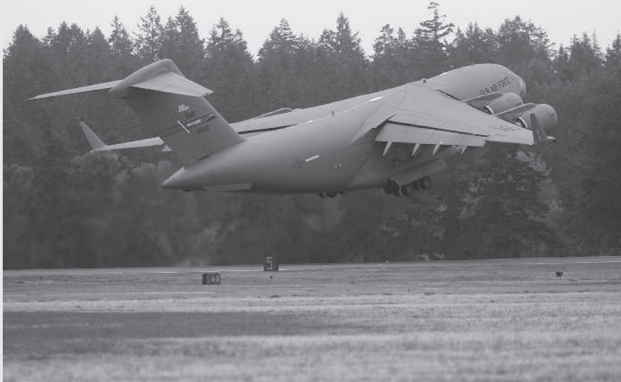
C-17 with wing flaps and leading-edge devices extended and winglets visible (U.S. Air Force photo by Abner Guzman)
