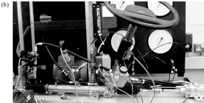
Figure 7.38. Test circuit for the analysis of a power-steering unit (Xue and Watton, 2005).
