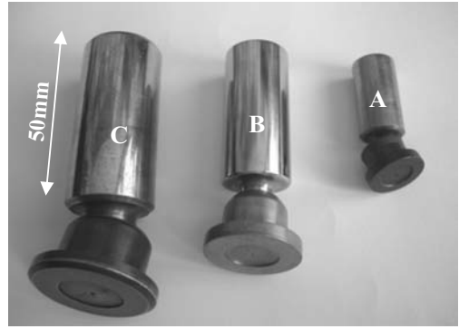
Figure 3.24. Three different piston sizes for an axial piston pump.
