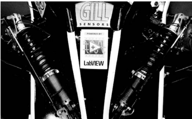
(b) Front MR dampers and position sensors
