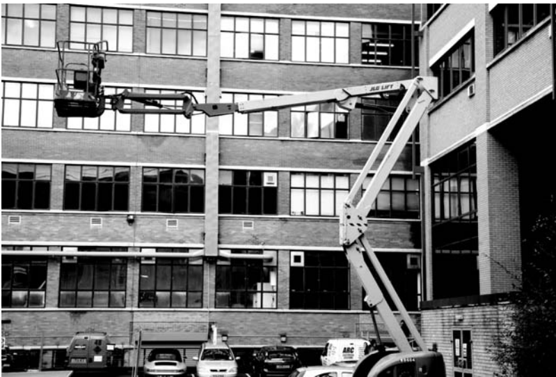
Figure 1.30. A mobile machine in a suspended condition using a pilot-operated check valve.
