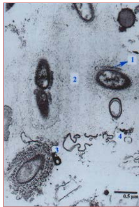
FIG. 4.8. – Transmission electron microscopy image of an activated sludge floc section showing bacterial cells embedded in mucoïd (1, 2) or capsular (3) extracellular polymeric substances (EPS) constituting the matrix of the aggregate. Some fragments evoke wall pieces (4) suggesting the presence of intracellular contents in the EPS matrix (from Bleich & Nehrkorn, 1989 [15]).
