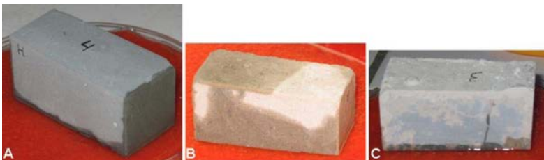
FIG. 13.1. – Capillary imbibition tests - skin effect and influence of cracking [18].
