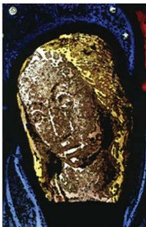
FIG. 15.15. – Browning on the surface of a fifteenth century stained glass window (Les Noës-Près-Troyes church, France).
