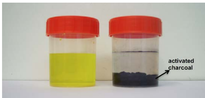
FIG. 1.1. – Solution of a yellow food dye, before (left) and after (right) treatment with activated charcoal particles, which were directly introduced in the solution.
