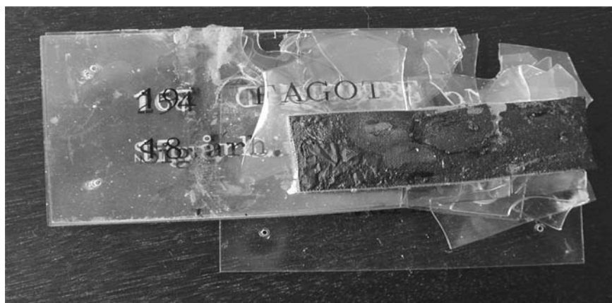
Figure 2 Poster made from cellulose nitrate in 1960s showing shrinkage due to loss of camphor plasticiser and cracking
