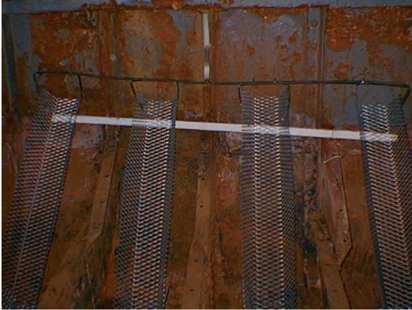
Figure 11 Stainless steel anodes used in the electrolytic conservation of M33
