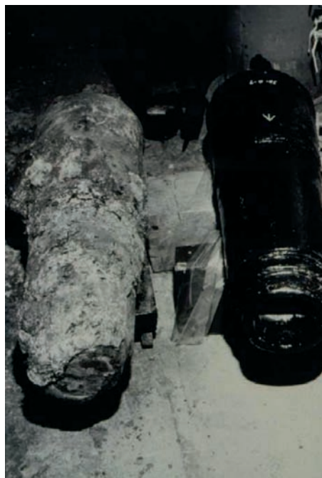
Figure 13 Similar caronades from HMS Pomone before and after conservation in the hydrogen furnace
