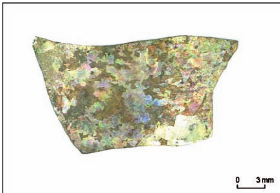
Figure 7 Fragment of an archaeological vessel glass damaged by "iridescence": a network of micro-cracks is covering the entire surface, which has already partly flaked off
