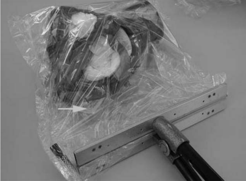
Figure 5 Rubber gas mask being enclosed with oxygen absorber (indicated by arrow). Bag is flushed with nitrogen just prior to closure by heat sealing
