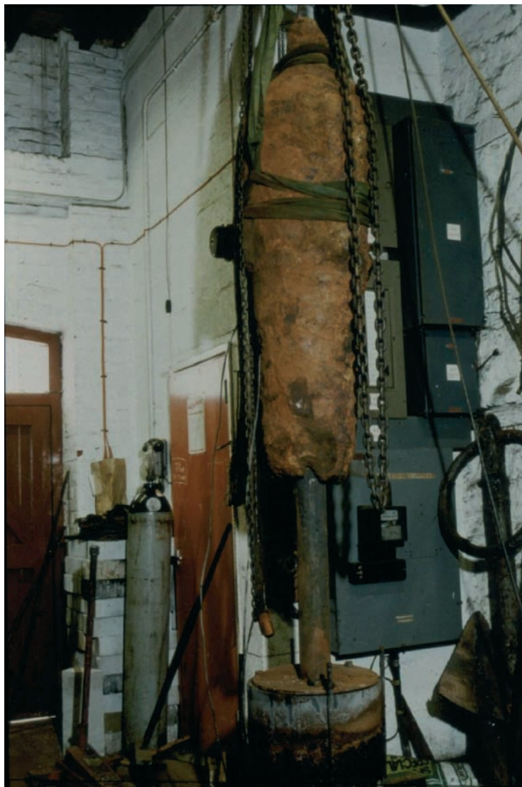
Figure 12 Loading a gun onto the retort of the hydrogen furnace
