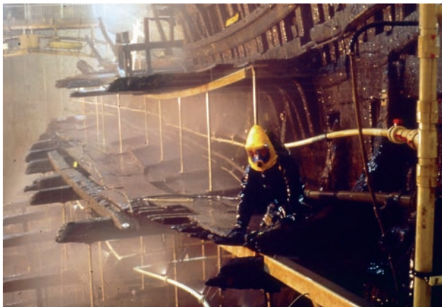
Figure 19 Spraying the hull timbers with a solution of PEG
