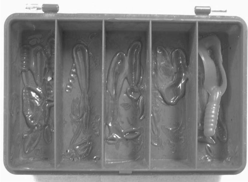
Figure 3 A polyethylene fishing-box has absorbed plasticiser from plasticised PVC lures and formed polyethylene 'fossils' over 20 years
