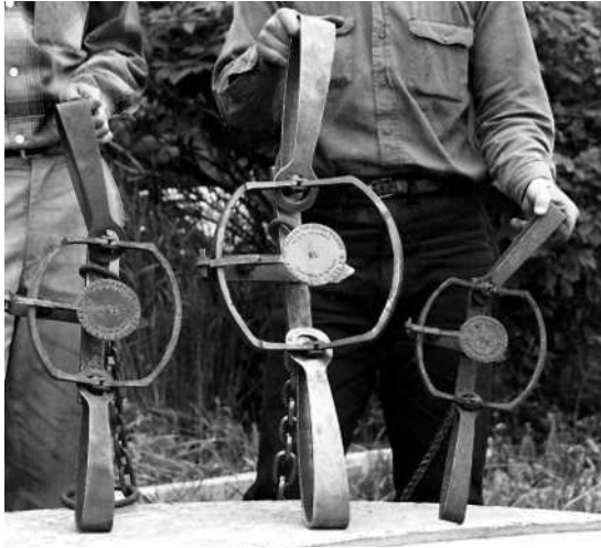
FIGURE 47 The #150 double-spring steel trap with offset jaws (left side) was effective for capturing bears.
