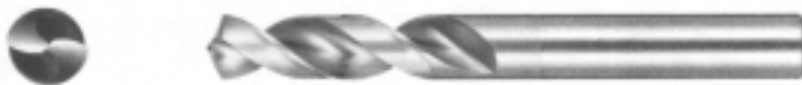
A520 – ADX stub length drill for NC and CNC machines, high productivity and accurate holes, special 130^\circ thinned point convex cutting lip, TiN coating
