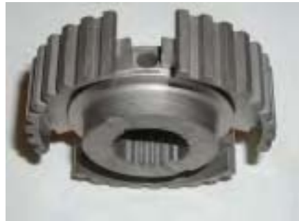
b – Synchronizer hub with 3 blind holes drilled \text{\O}5.5 mm (MIBA, Vorchdorf)
