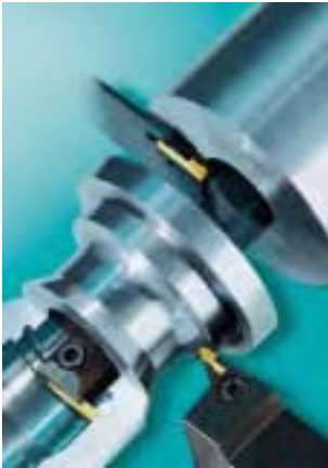
Fig.8.9 Illustrative view on curve and cut off turning of wrought steel bar.
