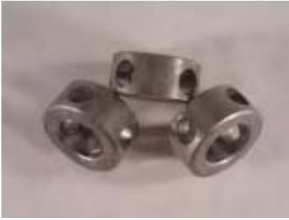
Fig.2.14 The specimens – rings cold compacted in one stroke in a rigid closed die from mixed alloyed powder with four cross through holes. (Courtesy of Institute of Materials Research of SAS, Košice).
