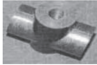
Fig.2.17 Threaded blind hole (M6) in cross-flow PM steel green part produced by WFC [16,17].
