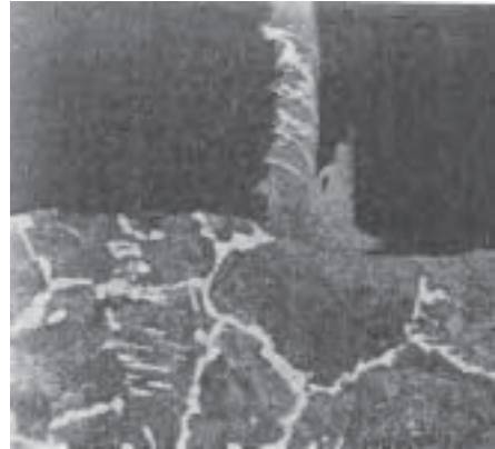
Fig.3.21 Schematic of cutting process with a built-up edge [112].
