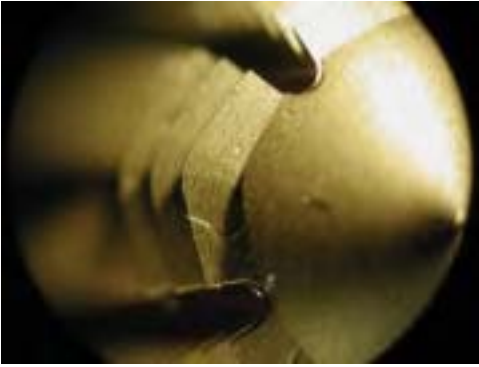
Fig.8.14 View on split point geometry of cold forming tap with flutes M8.
