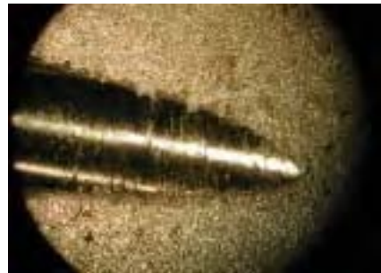
Fig.7.78 View of the failed cutting edges of a standard HSS 3 mm drill after drilling Cr-steel (Tab.7.28).
