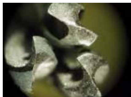
Fig.7.76 View on drill point - cutting edges of a new standard HSS 3 mm drill (left) and of HSCo 3 mm drill with modified geometry (right).
