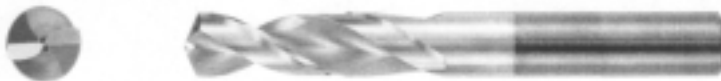
R520 – CDX micrograin hardmetal stub drill, 130^\circ special point convex cutting lip, TiN coating
