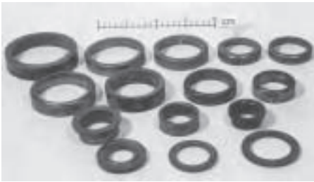
Fig.7.124 Powder forgings of bearing rings prepared from Astaloy A, and Sumirons 4100 S powder [23].
