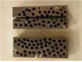
Fig.3.46 Two impact test bars as-clamped and as-separated after drilling test [153].
