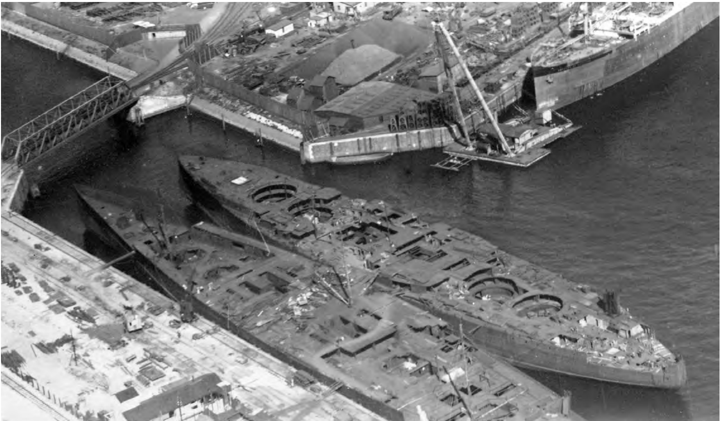
The incomplete Ersatz-Freya and Württemberg being broken up in the Roßhaven at Hamburg in late 1921. (AD collection)
