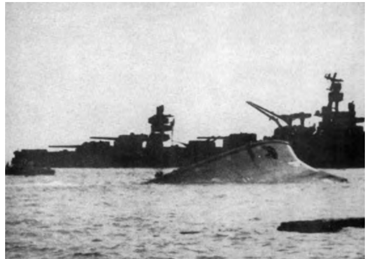
Sakawa at Bikini Atoll after Test Able on 1 July 1946; she had been moored 384 metres from the explosion and had most of her superstructure demolished; leaking badly, she sank the next day in spite of an attempt to tow her to a beach. Resting in some 60 metres of water, the wreck was further damaged in Test Baker, whose bomb was detonated underwater 150 metres away; the ship in the background is the battleship USS Arkansas , with her funnel demolished by the explosion. (Office of the Historian, Operation Crossroads, pp 162–3)
