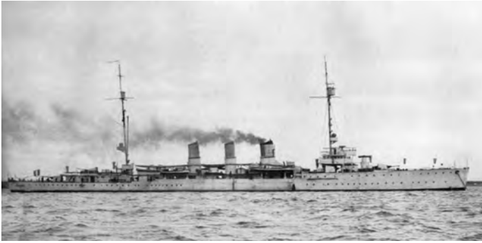
Taranto in July 1937, after her reconstruction and trunking of her forward funnels. (AD collection)
