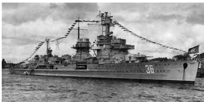
Admiral Makarov (ex- Nürnberg ), little altered from her German form, apart from a reduction in the size of her light AA battery and the fitting of new electronics. (AD collection)
