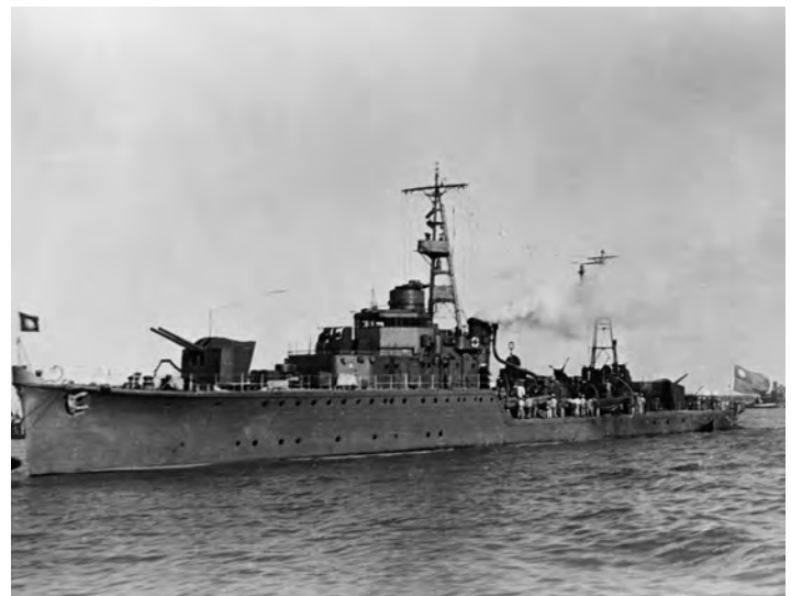
Chang Chi (ex- Uji ) in Nationalist service, rearmed with ex-coastal guns; she fell into Communist hands and, as Nan Chang , was again rearmed, this time with Soviet weapons. (NHHC NH 96191)
