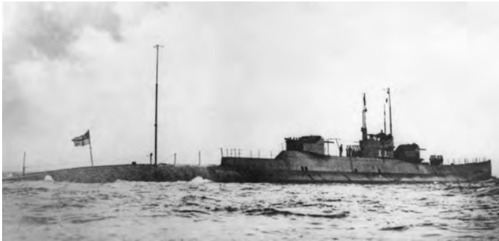
The British submarine-cruiser X1 , whose battery-chargers were powered by two 1,200bhp MAN diesels removed from U126 . (AD collection)
