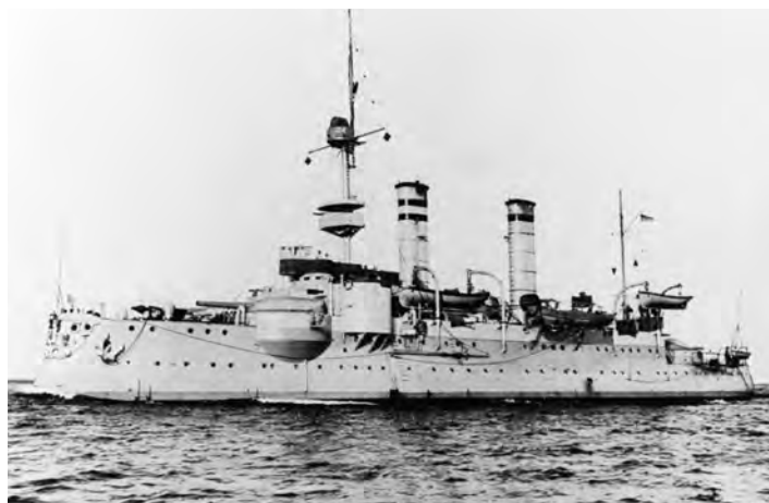
Odin , shown before and after her rebuilding from a coast defence vessel to a mercantile locomotive transport. Although converted to the same basic concept, Odin differed from her sister Aegir and half-sister Frithjof in having a single mast, rather than their two. (NHHC NH 47884; Drüppel)
