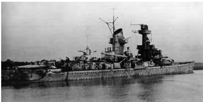
The wreck of Lützow , with 30m of her starboard side opened up by a near-miss by a 12,000lb ‘Tallboy’ bomb on 16 April 1945. She was also struck by three 1,000lb bombs: one of which had penetrated three decks; another two decks (albeit without exploding); and one that created a 6 x 1.5m hole in the upper deck. Righted from her heavily listed post-attack state, her forward turret remained in action until the hulk was further damaged by demolition charges by the retreating Germans on 3 May, including wrecking her main turrets. (AD collection)
