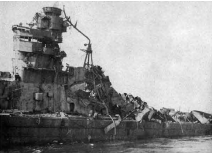
Sakawa at Bikini Atoll after Test Able on 1 July 1946; she had been moored 384 metres from the explosion and had most of her superstructure demolished; leaking badly, she sank the next day in spite of an attempt to tow her to a beach. Resting in some 60 metres of water, the wreck was further damaged in Test Baker, whose bomb was detonated underwater 150 metres away; the ship in the background is the battleship USS Arkansas , with her funnel demolished by the explosion. (Office of the Historian, Operation Crossroads, pp 162–3)
