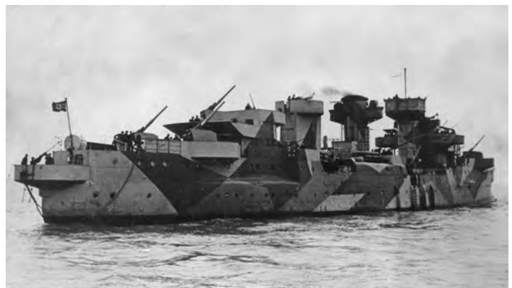
Arcona (shown here) and Medusa also became hulks, and were rebuilt as immobile anti-aircraft batteries during the Second World War. (AD collection)
