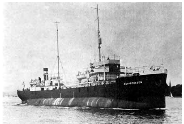
The tanker Ostpreussen , constructed around the pressure hulls of the unfinished submarines U183 and U184 . (AD collection)
