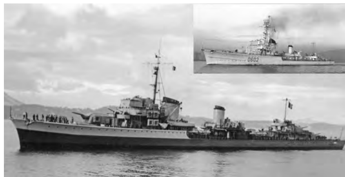
Hoche (ex-Z25) had already had no. 4 gun removed while in German service. She is shown here in 1948 before any substantive modifications, while serving in the 1st Destroyer Division at Cherbourg. She passed into reserve the following year, and was then extensively refitted during 1951–53, with her bridge enlarged, the twin turret forward replaced by a single mounting, eight 40mm guns installed in lieu of her original AA battery, and French 550mm TT replacing her German ones (see inset). (AD collection)
