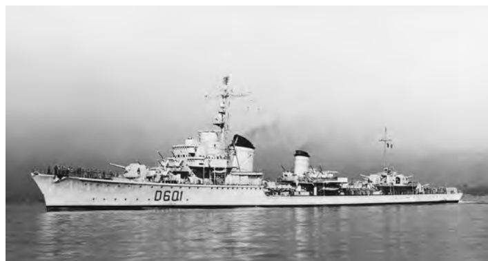
Marceau (ex-Z31) had been acquired with a single 105mm gun forward, temporarily replacing a destroyed 150mm twin mounting. However, during her 1948–50 refit, this was replaced by a single 150mm weapon, and eight 40mm guns installed in lieu of her German AA battery. (AD collection)
