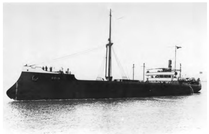
Odin , shown before and after her rebuilding from a coast defence vessel to a mercantile locomotive transport. Although converted to the same basic concept, Odin differed from her sister Aegir and half-sister Frithjof in having a single mast, rather than their two. (NHHC NH 47884; Drüppel)
