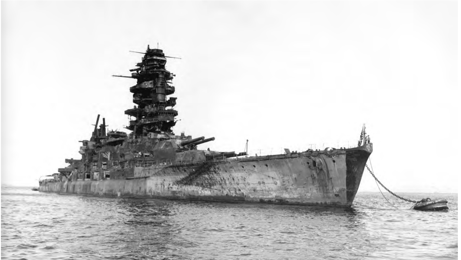
Nagato , pictured here on 9 September 1945, had been reduced to an anti-aircraft battery at the beginning of the year, with the upper part of her funnel and mainmast cut away to clear sky arcs, and her secondary battery landed in two phases. Power was provided from ashore and a sub-chaser moored alongside. She was damaged by two 500lb bombs on 18 July, but remained afloat, the last Japanese battleship. (AD collection)
