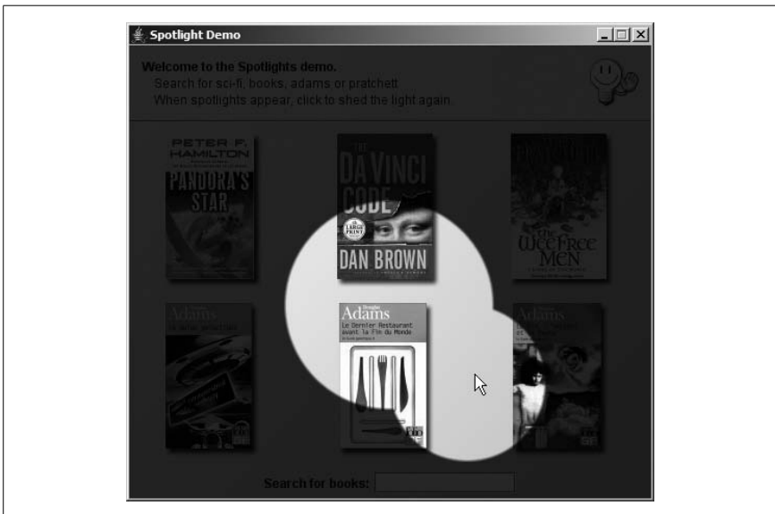
Figure 8-15. By subtracting ellipses to a rectangle, you can easily overlap the spotlights
