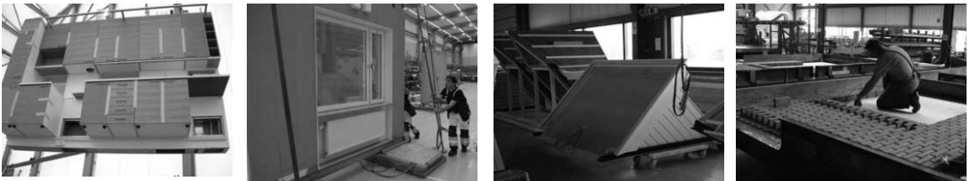
Figure 4 Examples of fabrication of modules and subsystems (NCC and Burggraaf)
