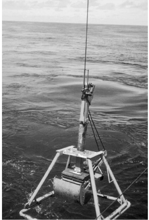
Figure 9. Box corer for collecting a large volume of sediments. Courtesy A. B. Valsangkar, Geological Oceanography Division, National Institute of Oceanography, Dona Paula, Goa, India.
