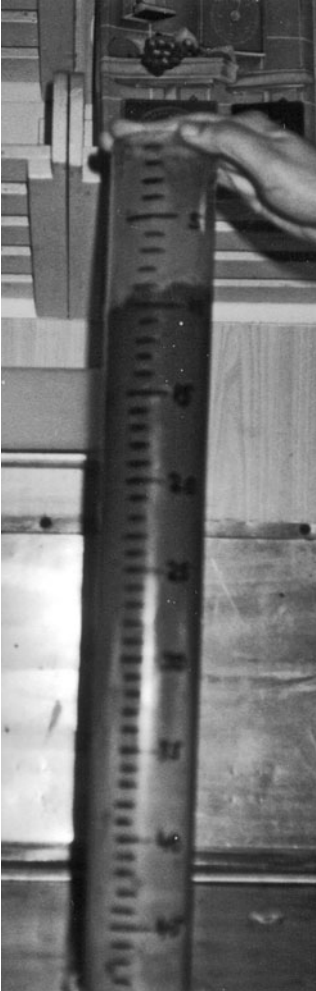
Figure 10. A graduated polyvinyl chloride cylinder for collecting sediment subsamples from a box corer. Courtesy A. B. Valsangkar, Geological Oceanography Division, National Institute of Oceanography, Dona Paula, Goa, India.
