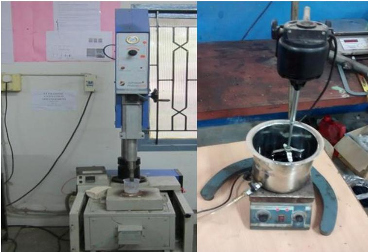
Figure 2. Ultrasonic agitator and mechanical stirrer arrangement.
