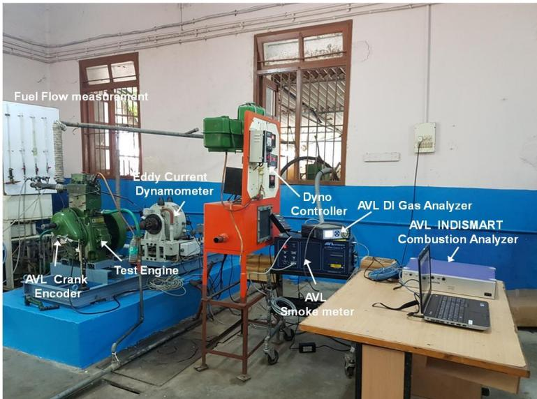
Figure 3. Photographic view of the test engine setup.
