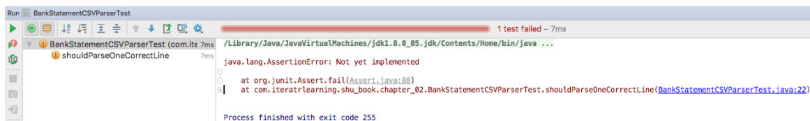
Figure 2-2. Screenshot from the IntelliJ IDE of running a failing unit test
