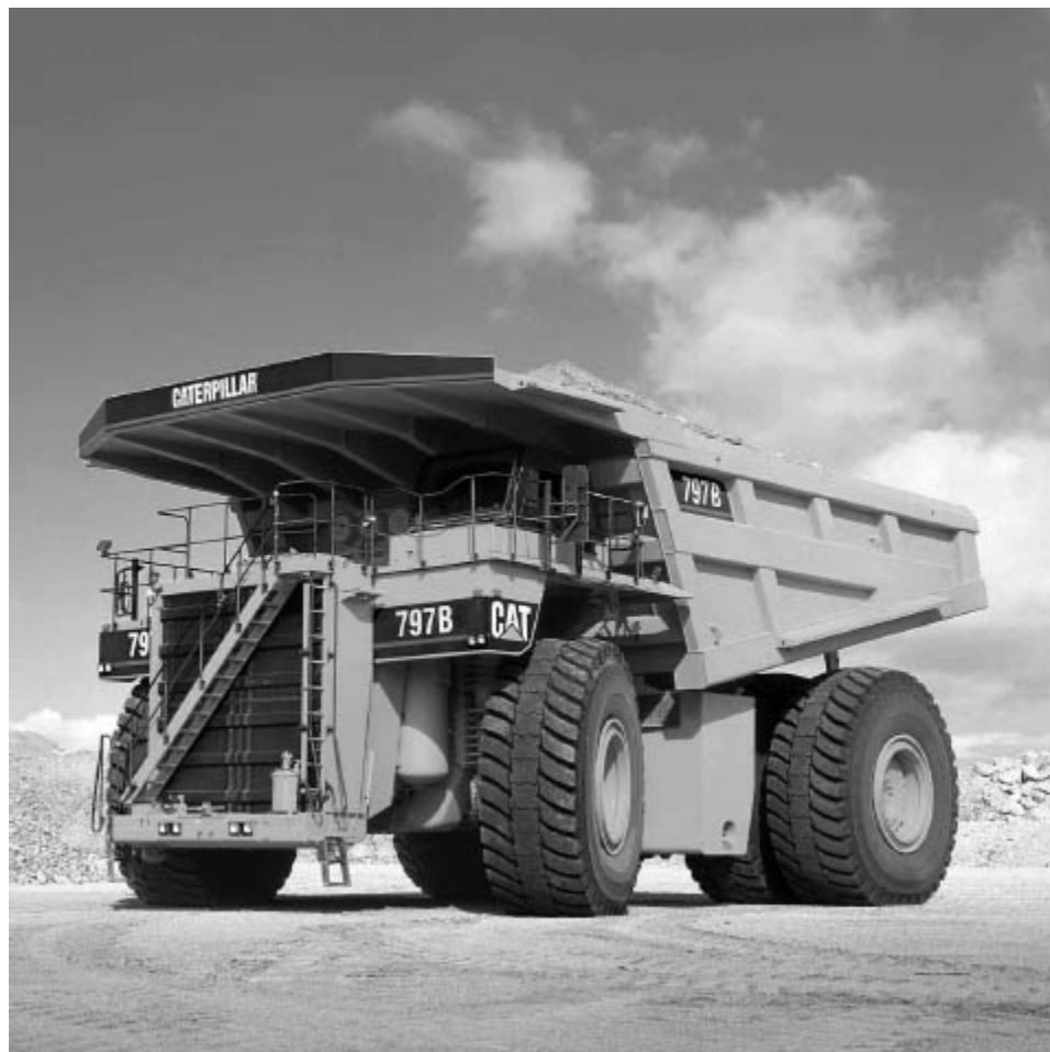
Figure 5.17 Caterpillar's largest off-road truck, the 797B. Photograph available at the Caterpillar Web site.
