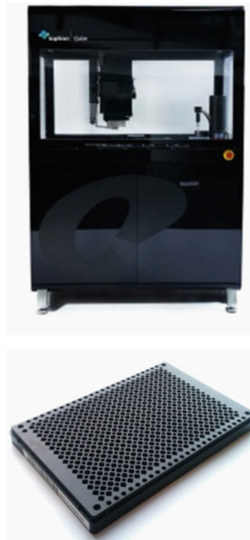
Fig. 2 Qube 384 (top) and the QChip 384 measurement plate (bottom)
