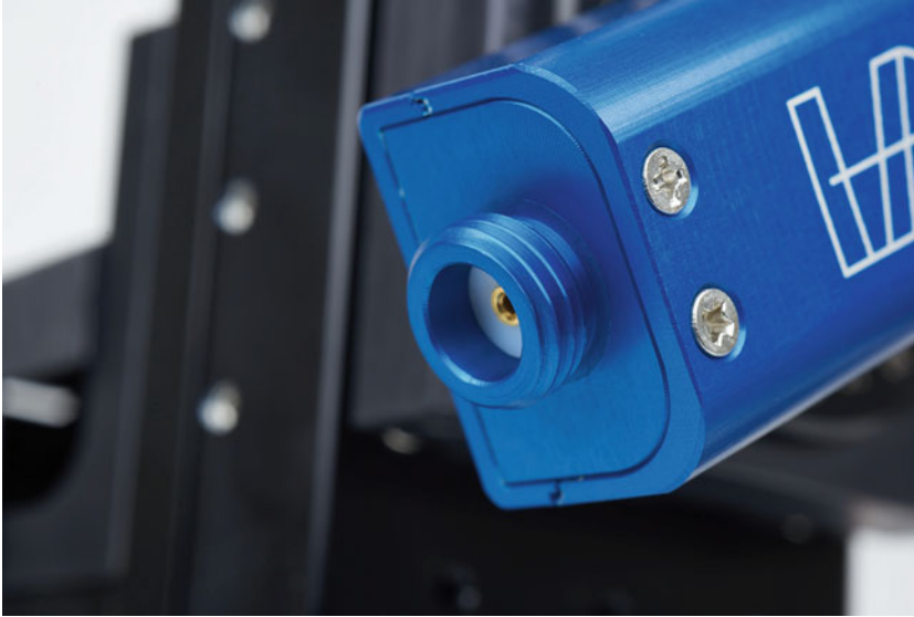
Fig. 1 The pipette holder fitting on Sutter Instrument amplifiers is compatible with Axon Instruments' HL-U standard, which has been adopted by several other manufacturers. The threaded collar on Sutter headstages is executed in metal rather than the commonly used Teflon ® . This provides both greater mechanical stability and better electrical shielding
