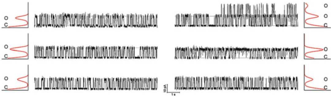
Fig. 7 Parallel single-channel recordings on the MECA-16 chip with corresponding all points histograms showing current distribution for in vitro-translated KcsA E71A channels reconstituted via proteoliposome fusion. Gray lines indicate the channel open (O) and closed (C) states respectively. KcsA E71A was translated in the presence of Asolectin liposomes, which were subsequently enriched with POPG lipids and fused with POPE–POPG (3:1) bilayers on the MECA-16 chip. V_{\text{hold}} = 100 mV. Recorded in symmetric solution containing 200 mM KCl and 20 mM MES, pH 4.5 on the cis -side and 10 mM MOPS pH 7.5 on the trans side of the bilayers
