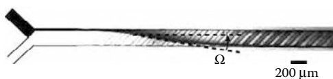
FIGURE 3.41 Optical micrograph taken from above of a stream of black dye flowing in a microchannel containing square grooves in the bottom of the channel. A narrow stream of black dye in water is injected alongside a broad stream of clear water (flow rate of the clear stream is 20 times that of the dyed one). The average flow speed in the channel is 1 cm/s (Reynolds number Re \sim 1 ) [471]. Reprinted with permission from the American Chemical Society.
