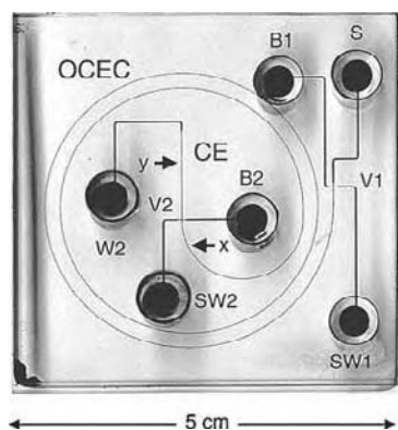
FIGURE 4.16 Image of the glass microchip used for 2D chemical separations. The separation channel for the OCEC (first dimension) extends from the first valve V1 to the second valve V2. The CE (second dimension) extends from the second valve V2 to the detection point y. Reservoirs for sample (S), buffer 1 and 2 (B1, B2), sample waste 1 and 2 (SW1, SW2), and waste (W2) are positioned at the terminals of each channel. The arrows indicate the detection points in the OCEC channel (x) and CE channel (y) [333]. Reprinted with permission from the American Chemical Society.
