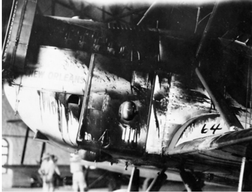
Erik Nelson and John Harding in the New Orleans nearly had a forced landing when an engine connecting rod broke splattering oil over the plane during the flight from Multan to Karachi, India. Nelson was able to nurse the plane for nearly an hour to a safe landing. (Photo: U.S. Air Force)
