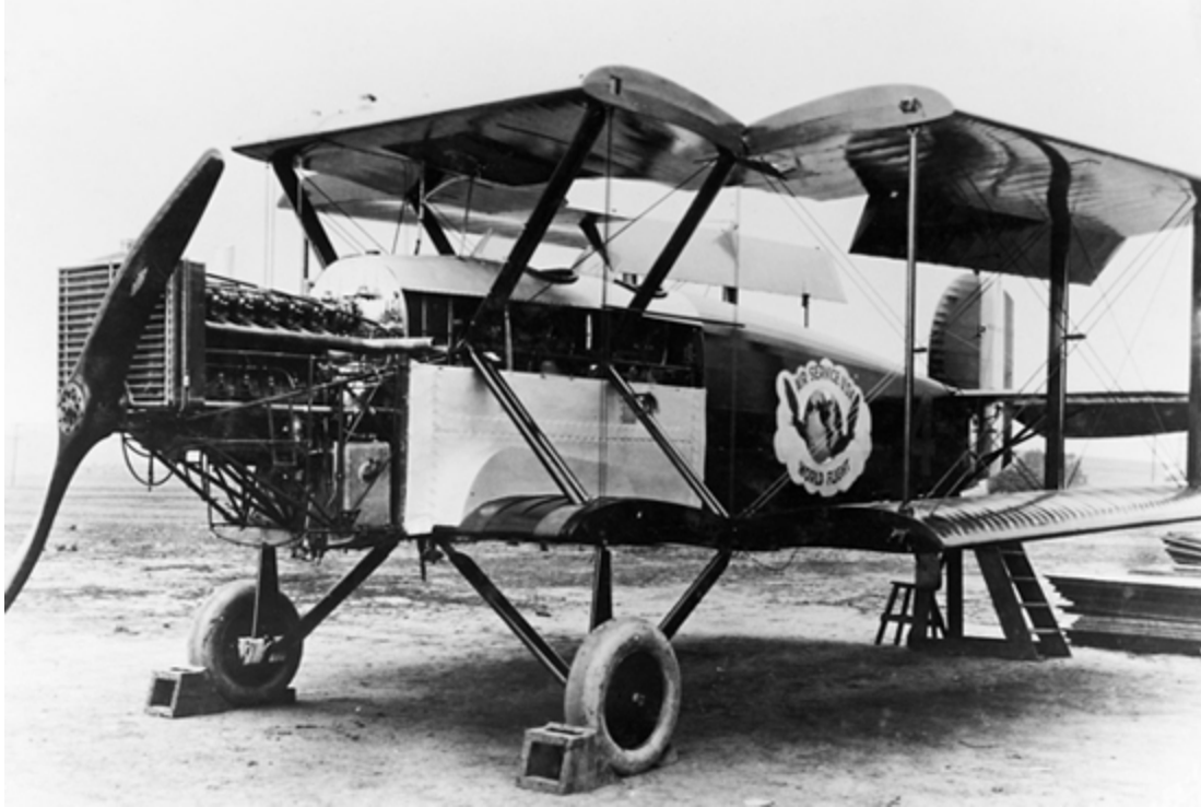
Three-quarter front view shows wings folded and engine without the cowling. The engine had two types of coolers: one for hot climates and a smaller one for arctic flying. (Photo: McDonnell Douglas Company)
