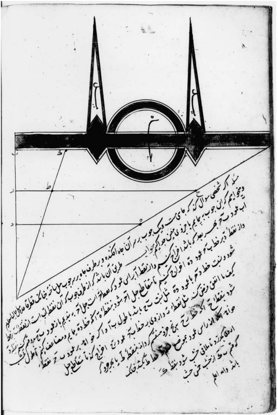
Fig. 6. The method of constructing an irrigation canal. From an anonymous compendium of works on astronomy, geometry, and mathematics. Iran, ca. 16th century. [Majmū'a], "Recueil d'ouvrages d'astronomie et de mathématiques." MS, Bibliothèque nationale de France, Ancien fonds persan 169, fol. 173b. Reproduced by permission.
