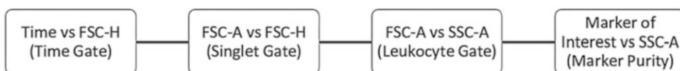
Fig. 4 The gating strategy employed to identify single markers and their purity. All created plots should be in dot plot format
