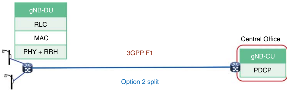
Figure 7.4 Single-level split NG-RAN architecture suitable for mmWave frequencies.
