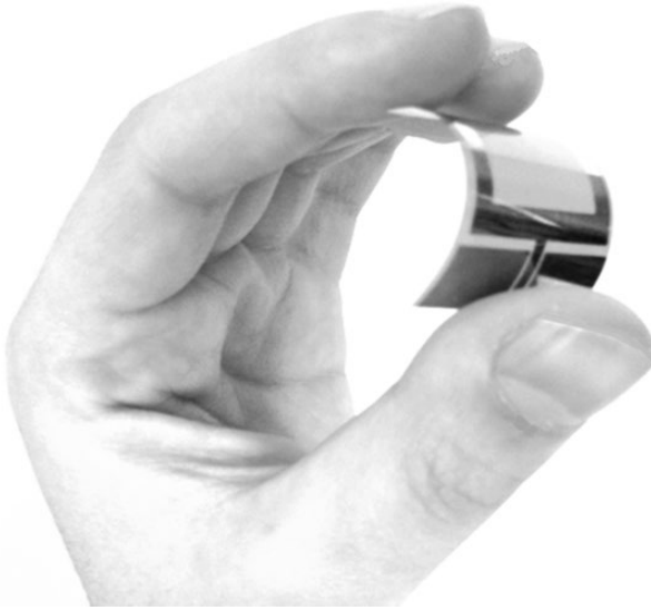
Figure 4.4 Printed monopole antenna intended for integration within flexible electronics.
