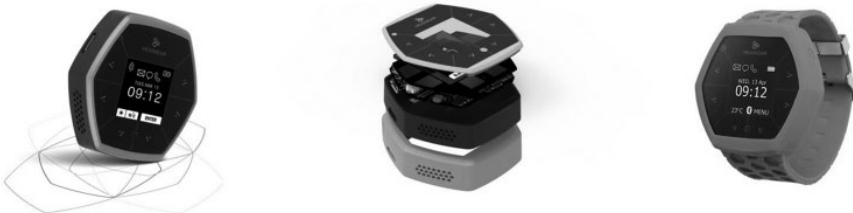
Figure 10.19 Hexiwear wearable development board. Source: Photo courtesy of MikroElektronika.
