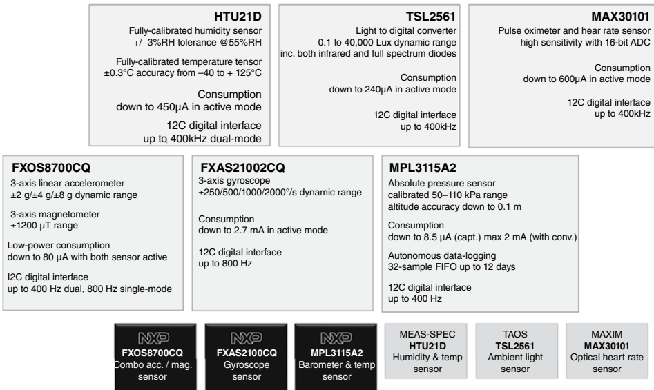
Figure 10.23 Hexiwear sensors specification and communication interfaces. Source: Courtesy of ARM.
