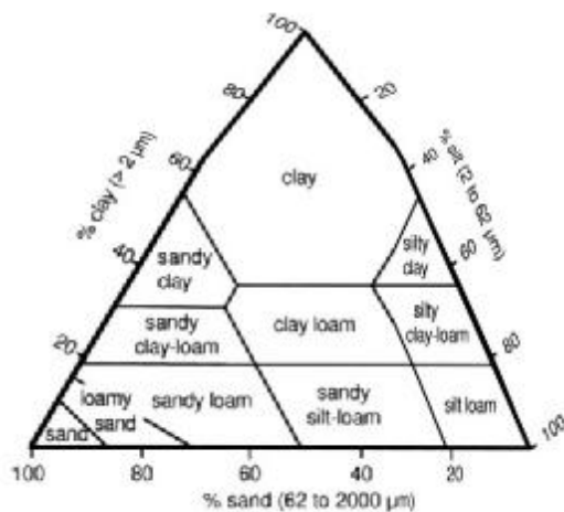
Figure 12.2. Ternary diagram to show the basic classes of sediment texture used in soil science (after Courty et al., 1989:37).
