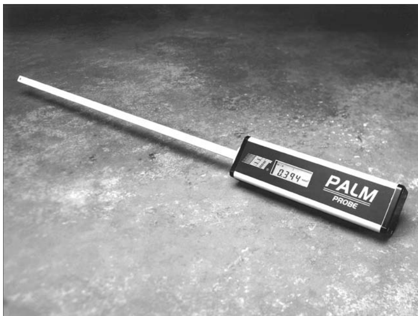
FIGURE 9.10 Probe for production ambient light measurement. (Courtesy of EIT, Inc.)
