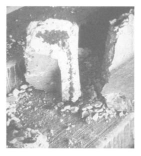
**Fig. 2.7.** The result of a phenolphthalein solution test on a fragment of concrete to establish the depth of carbonation.
