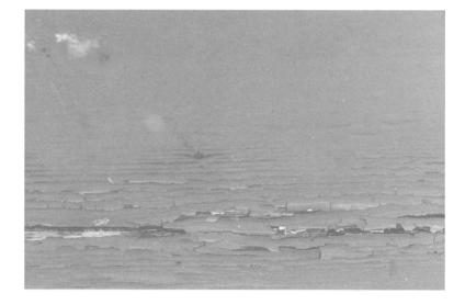
froths the paint, and small bubbles are created in the wet surface. These dry more rapidly than the surrounding film and the bubbles become trapped in the finished coating.
