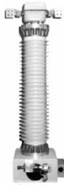
Figure 6.9 A commercially available optical current and voltage sensor. To meet existing standards, the optical outputs are converted to provide nominal outputs of 1A and 120V.
