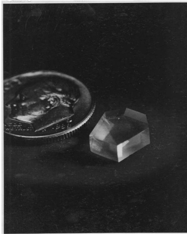
Figure 2.2 Photograph of the monolithic nonplanar Nd:YAG ring laser, NPRO, that operates in a single frequency with a linewidth less than 10 kHz. (After: [9].)
