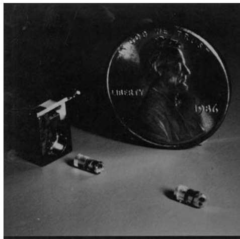
Figure 2.1 Photograph of the three elements of the first laser diode-pumped Nd:YAG laser constructed at Stanford. The laser operated with 2 mW of output power at 25% slope efficiency. (After: [8].)
