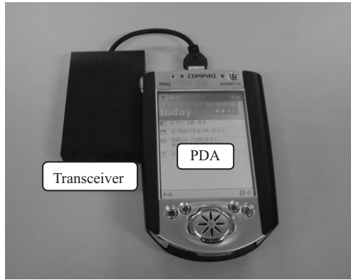
Figure 10.10 Photograph of the transceiver connected to a PDA.
