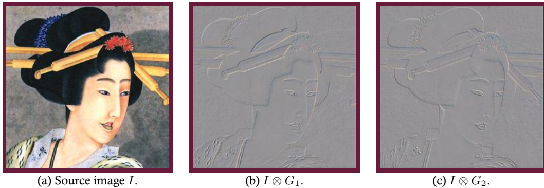
Figure 6.16. A source image is convolved with the Roberts operators G_1 and G_2 .
